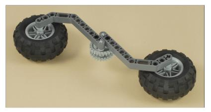
**Note:** After completing this step, you should check again to make sure that all of the parts spin easily. You should be able to spin the set of three tires, and they should coast easily by themselves in all three different gear positions. You should also now be able to shift gears using the shift lever if the tires are turning.
